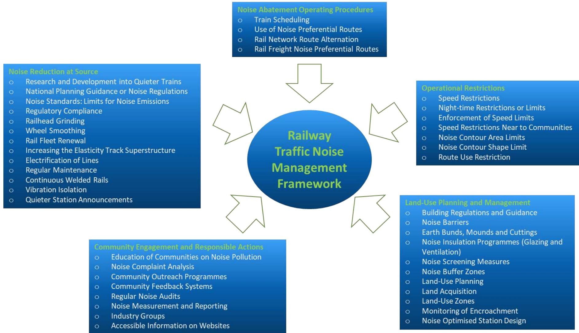
Figure 16: Railway Traffic Indicative Noise Management Framework
